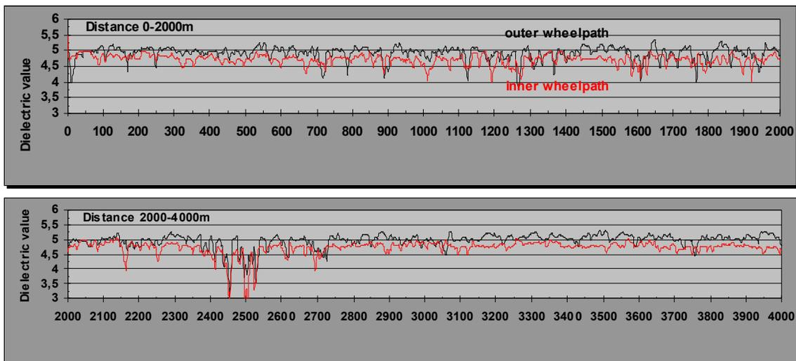
Figure 6. Dielectric value of asphalt in E4 at Ylinampa, north of Rovaniemi in Finnish Lapland. A reduction in dielectric value was observed at the end of each truckload and other places where an experimental paver had problems. The experimental paver was replaced by a conventional machine at 2700 m and after that the quality immediately improved.
