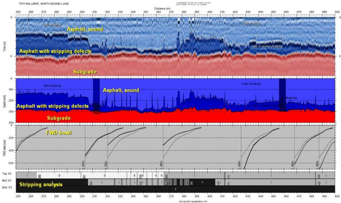
Figure 7. A 1.5 GHz ground coupled GPR profile, interpretation, falling weight deflectometer data and stripping evaluation from TH71 at Willmar, Minnesota. The slightly better section between 310 and 380 m can be seen also as better FWD deflection bowls.
