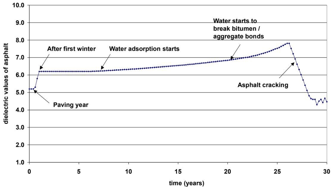
Figure 2. A schematic model of the dielectric history of an asphalt pavement.
