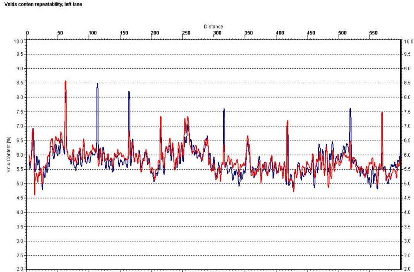
Figure 5. Repeatability of voids content. Two separate runs measured from the left lane. Voids content calculation reference point is from 257 m, where the voids content from the drill core was 7.3 %. The peaks are due to metallic sensors on pavement.
