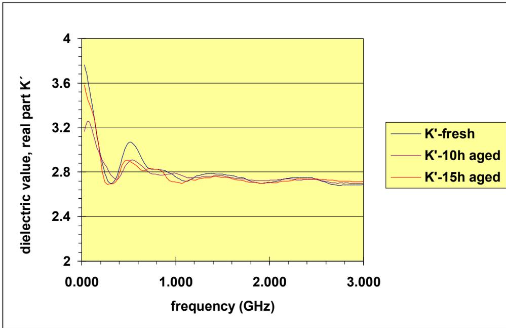
Figure 1. Real part  $K'$  of the dielectric value of Laguna bitumen when fresh and when aged using thin film oven test device.
