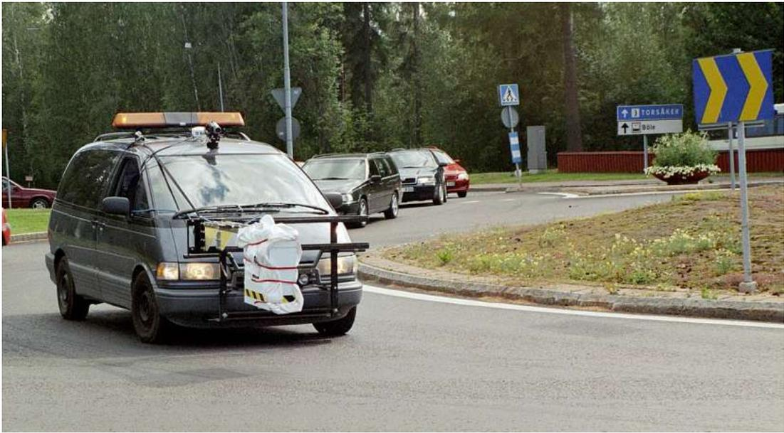
Figure 3. A GPR horn antenna system.
