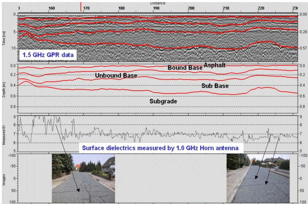
Figure 8. Detecting road sections with stripping problems in Wertlingen Germany. High surface dielectric values present the area where the stripped asphalt is saturated with water.
