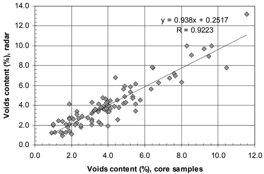
Figure 4. Correlation between voids content measured using the GPR technique and voids content from drill cores.
